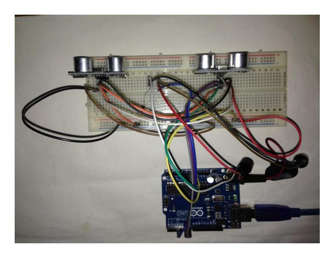
We connect a jumper wire from the 5 volt pin on the Arduino to the bottom channel of the breadboard
